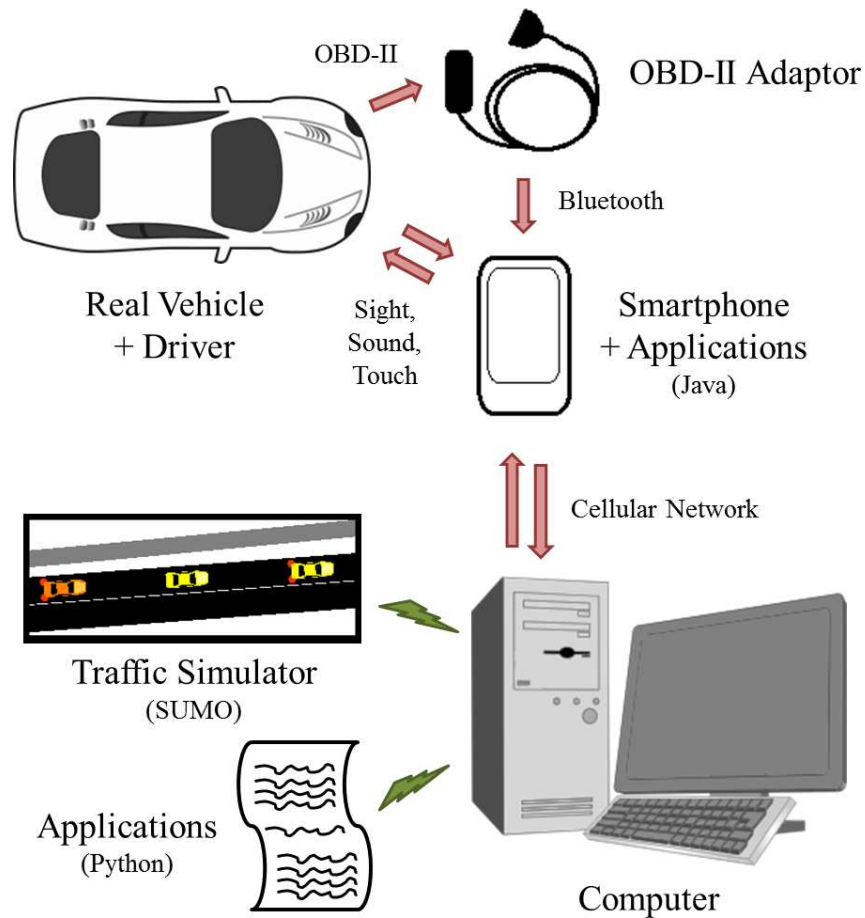
Fig. 1 Illustration of the VIL platform setup described in [12]. In [12], the essential notion was that ITS applications were deployed on the workstation computer also interfacing hundreds of vehicles in SUMO, while a corresponding application was deployed on the smartphone which served as the interface to the driver and the real vehicle. The simulated vehicles, and the real vehicle, both provided inputs for the control algorithms and applications to be tested. (The real vehicle and computer sub-images contained within this illustration were downloaded from https://openclipart.org on 27 July 2016 and 22 September 2017, respectively.)
